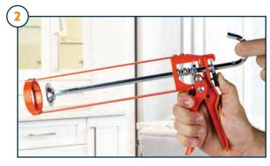
Never hold the applicator as shown above. The push rod cannot be withdrawn whilst the trigger is depressed – even slightly. Any pressure on the trigger will lock the push rod in place.
